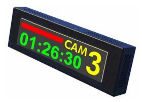
Tekskil's latest and most powerful tally display is our TallyCLOCK©. This display combines dual mode tally, camera ID and clock. The clock operates in three modes; a slave SMPTE VITC Time Code display, direct feed from the Studio Master Clock or Time of Day with time zone offset. The TallyCLOCK is a custom LCD panel that enables customization of size, position, color and brightness of every display function - the ultimate in tuning display mode to the needs of the talent.
